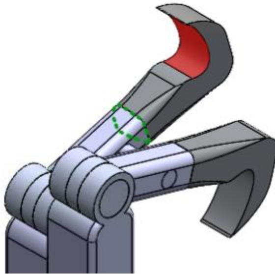
Figure 16: Force was applied normally to the red surface. The geometry outlined in green dotted lines was held fixed.
